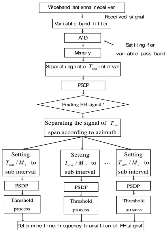
Figure1. Detection Block Diagram of FH signal using PSDP
